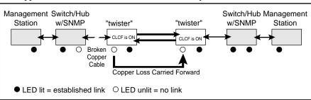
Loss of link at the fiber port is not propagated, as shown in the example below.
